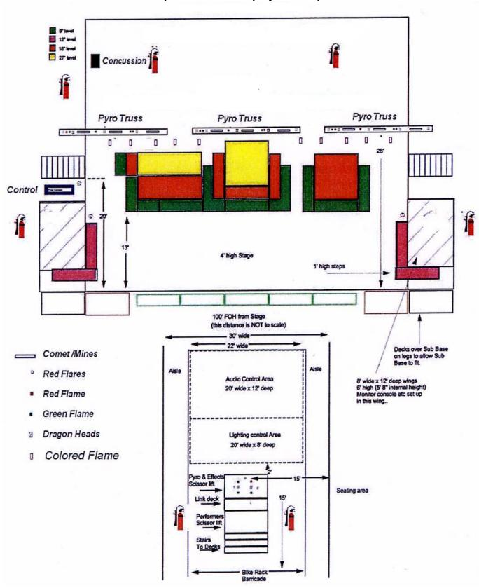
Permit and Plan Submittal Requirements for Firework, Pyrotechnic and Flame Effect Productions Example of Indoor Display Site Map
